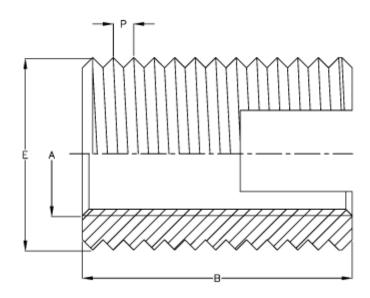
Female thread A = M4Length B = 6Male thread E = 6.0Min hole depth blind hole = 8Recommended bore diameter (hard mat.) = 5.5 to 5.6Recommended bore diameter (soft mat.) = 5.3 to 5.4Thread pitch P = 1.00Type  $= 303 \ 0 \ 040.$
